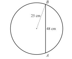
A frame consists of a uniform circular ring of radius 25 cm and mass 1.5 kg, and a uniform rod of length 48 cm and mass 0.6 kg. The ends *A* and *B* of the rod are attached to points on the circumference of the ring, as shown in the diagram. Find the distance of the centre of mass of the frame from the centre of the ring. [4]
