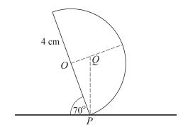
A uniform solid hemisphere, with centre O and radius 4 cm, is held so that a point P of its rim is in contact with a horizontal surface. The plane face of the hemisphere makes an angle of 70° with the horizontal. Q is the point on the axis of symmetry of the hemisphere which is vertically above P. The diagram shows the vertical cross-section of the hemisphere which contains O, P and Q.
