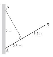
A uniform beam AB has length 6 m and mass 45 kg. One end of a light inextensible rope is attached to the beam at the point 2.5 m from A. The other end of the rope is attached to a fixed point P on a vertical wall. The beam is in equilibrium with A in contact with the wall at a point 5 m below P. The rope is taut and at right angles to AB (see diagram). Find
